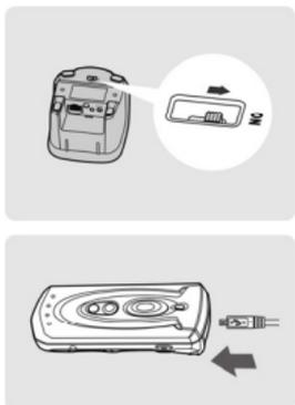
The scanner can also be charged via the USB 3.0 port without the power supply unit. You can connect the cradle to USB 3.0 port of host device by a USB cable, then slide the USB bus power switch to “ON”. After that, place the scanner onto the cradle.
